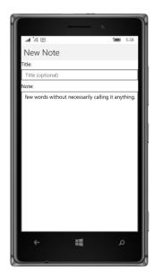
It is not necessary to enter a title. If there is none, an identifier is constructed that consists of the beginning of the text. Nor is it necessary to enter the note text. A note can consist solely of a title. (At the time this chapter was written, the Windows Runtime Editor didn't properly wrap text.)
