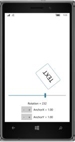
The iOS screen shows rotation around the center of the element (which is always safe on iOS despite the Anchorx and Anchory bug), while the rotation on the Android screen is around the upper-left corner, and the rotation on the Windows 10 Mobile screen is centered on the bottom-right corner.
