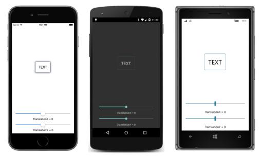
You can manipulate the sliders to move the Frame around the screen. The values of TranslationX and TranslationY specify an offset of the element relative to its original layout position:
