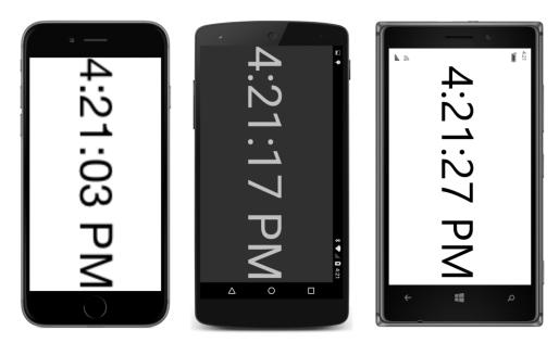
And here you can detect a little difference in the implementation of the Scale property in iOS compared with Android and the Windows Runtime. On Android and Windows, the resultant text looks as though it were drawn with a large font. However, the text on the iOS screen looks a little fuzzy. This fuzziness occurs when the operating system *rasterizes* the prescaled Label, which means that the operating system turns it into a bitmap. The bitmap is then expanded based on the Scale setting.
