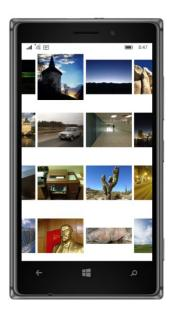
The Image elements load the bitmaps in the background, so the WrapLayout class will get numerous calls to its Layout method as each Image element gets a new size based on the loaded bitmap. Consequently, you might see some shifting of the rows and columns as the bitmaps are being loaded.
