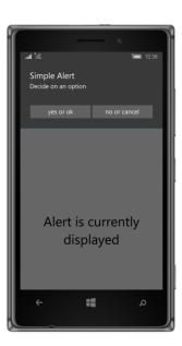
Of course, the alert essentially disables the user interface of the application, but the application could still be doing some work while the alert is displayed. For example, the program could be using a timer, and that timer would continue to run. You can prove this to yourself by adding the following code to the constructor of the **AlertCallbacks** code-behind file:
