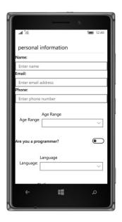
Even though the IsProgrammer switch is off, and the IsEnabled property of each of the last two PickerCell elements is set to false, those elements still respond and allow selecting a value. Moreover, the PickerCell doesn't look or work very well on the Windows 10 Mobile platform.
