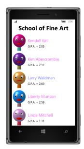
Something quite similar can be done with a data binding directly from the Sex property of the Student object to the TextColor property of the Label (or the ImageCell), but it would require a binding converter. The DataTrigger does the job without any additional code.
