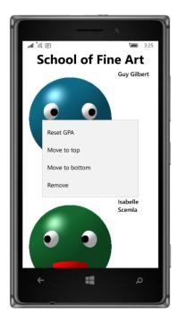
Only one menu item appears on the iOS screen, and that's the item that removes the student from the list. A menu item that removes an entry from the ListView must be specially flagged for iOS. The Android screen lists the first two menu items at the top of the screen. Only the Windows Runtime lists them all.
