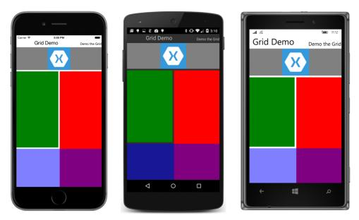
The screenshots confirm that the first row is sized to the height of the large Label; the second row is 100 device-independent units tall; and the third and fourth rows occupy all the remaining space. The third row is twice as tall as the fourth. The two columns are equal in width and divide the entire Grid
