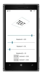
You'll discover that the Anchory property affects RotationX but not RotationY. For the default Anchory value of 0.5, RotationX causes rotation to occur around the horizontal center of the visual object. When you set Anchory to 0, rotation is around the top of the object, and for a value of 1, rotation is around the bottom.
