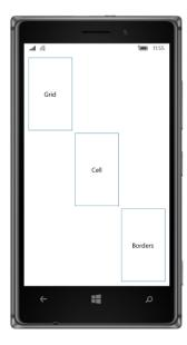
It might be a little disconcerting that the corners of the borders don't meet, but that's due to the default row and column spacing of the Grid. Set the RowSpacing and ColumnSpacing attributes to 0, and the corners will meet although the lines will still seem somewhat discontinuous because the borders are in different cells. If this is unacceptable, use the technique shown in **GridCellDividers**.
