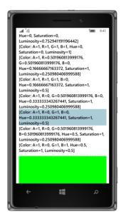
Actually, it's hard to tell whether that really is the "Lime" entry without examining the RGB values. Although the Color structure defines a bunch of static fields with color names, Color values themselves are not identifiable by name. When the data binding sets a Lime color value to the SelectedItem property of the ListView, the ListView probably finds a match among its contents using the Equals method of the Color structure, which compares the components of the two colors.
