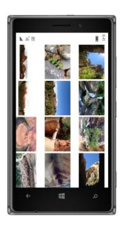
The ScrollView allows the layout to be vertically scrolled. If you want to check the different orientation of the WrapPanel, you'll need to change the orientation of the ScrollView as well:
