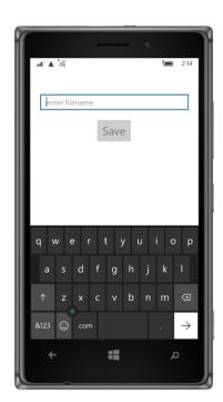
Although this represents a tiny enhancement to the user interface, if you didn't have a DataTrigger you'd need to implement this enhancement in code in a TextChanged handler of the Entry, or you'd need to write a binding converter for a Binding between the IsEnabled property of the Button and the Text.Length property of the Entry.
