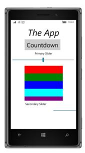
The TranslateTo call uses the Easing.SpringOut function, which means that each animated element should overshoot its destination and then move backward to come at rest in the center of the page. However, you won't see this happen. As you've already discovered, the TranslateTo method stops working when an easing function has an output that exceeds 1.
