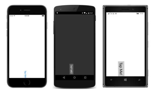
Now let's make the Button keel over and land upside down, which means that we want to rotate the Button around the upper-right corner. This requires a change in the AnchorX and AnchorY properties:
