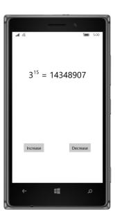
Once again, the wisdom of separating the user interface from the underlying business logic is revealed when the time comes to change the View. For example, suppose you want to replace the buttons with an element with a TapGestureRecognizer. Fortunately, TapGestureRecognizer has a Command property:
