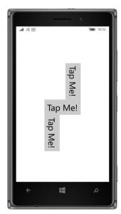
When we set new values of AnchorX and AnchorY, we need to adjust the TranslationX and TranslationY properties so that the Button essentially moves from the rotated position in the upper-right to the rotated position in the lower-left. TranslationX needs to be decreased by the width of the Button and then increased by its height. TranslationY needs to be increased by both the height of the Button and the width of the Button. Let's try that:
