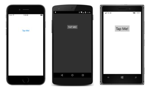
Recall that the Anchorx and Anchory properties must be set to numbers that are relative to the width and height of the Button. An Anchorx value of 0 refers to the left edge of the Button and a value of 1 refers to the right edge. Similarly, an Anchory value of 0 refers to the top of the Button and a value of 1 refers to the bottom.
