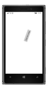
A second BezierPathTo then reverses the trip back to the upper-left corner. (This is where the BezierTangent enumeration comes into play. Without it, the Button suddenly flips upside down as the second BezierPathTo begins.) A final RotateTo restores it to its original orientation.
