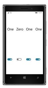
The saving and retrieving of program settings is handled in the code-behind file. Notice the handler assigned to the Toggled events of the Switch elements. The sole purpose of that handler is to store the settings in the Properties dictionary—and to save the Properties dictionary itself by using SavePropertiesAsync—whenever one of the Switch elements changes state. The dictionary key is the index of the Switch within the Children collection of the Grid:
